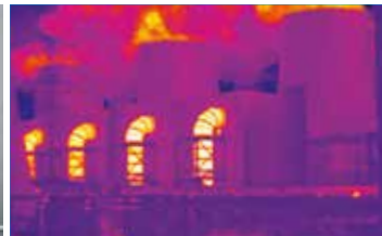
Heat leakage in a steam installation due to insufficient insulation.
